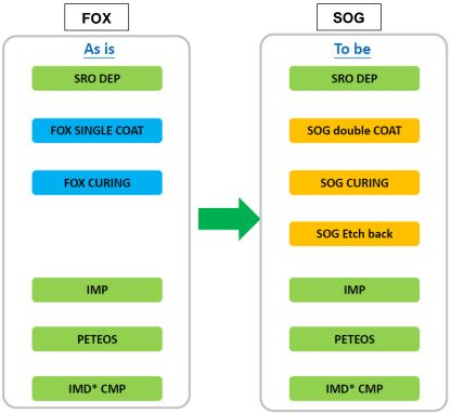
FOX no need to the etch back due to the cage structure
