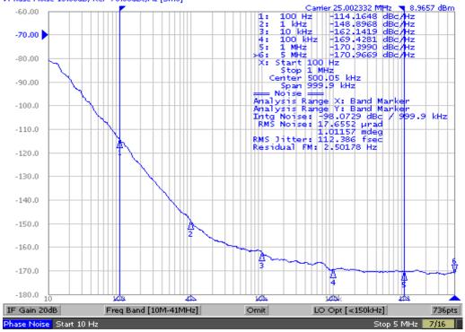
2.5V Core/2.5V Output RMS phase jitter (Random) 100Hz to 1MHz =0.112ps (typical)
