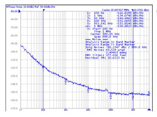
1.5V Core/1.5V Output RMS phase jitter (Random) 100Hz to 1MHz =0.277ps (typical)
