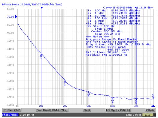
3.3V Core/3.3V Output RMS phase jitter (Random) 100Hz to 1MHz =0.098ps (typical)
