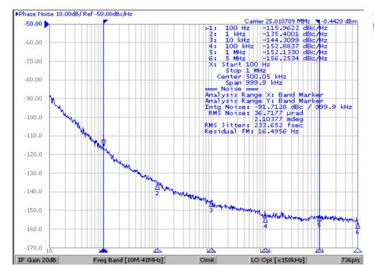
1.8V Core/1.8V Output RS phase jitter (Random) 100Hz to 1MHz =0.233ps (typical)
