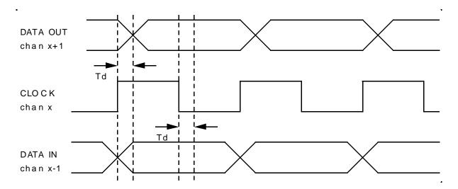
Figure D-29 SIOP Function Data Transition Example
