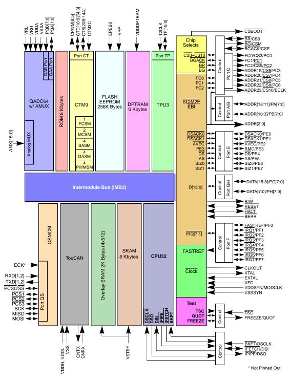
Figure 1-1 MC68F375 Block Diagram
