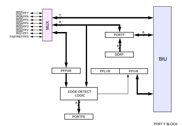
Figure 4-24 Port F Block Diagram
