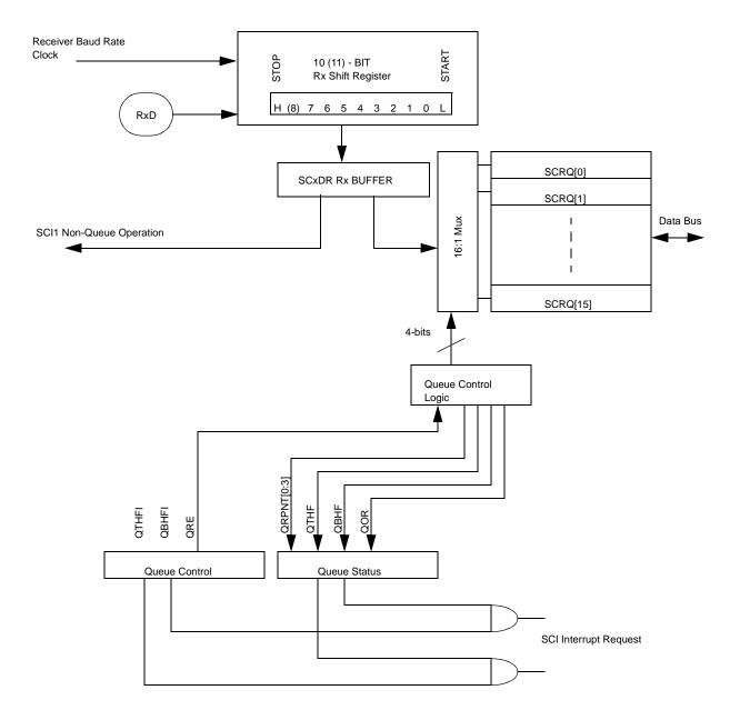
Figure 6-17 Queue Receiver Block Enhancements
