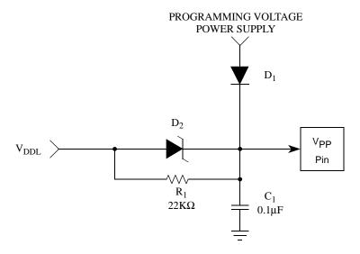
Figure E-23 A Recommended External V<sub>PP</sub> Pin Conditioning Circuit
