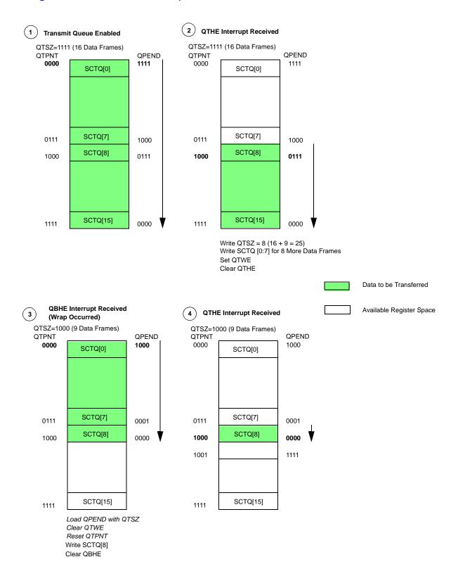
Figure 6-16 Queue Transmit Example for 25 Data Frames
