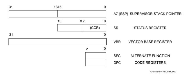
Figure 3-3 Supervisor Programming Model Supplement
