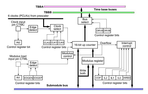
Figure 13-3 MCSM Block Diagram
