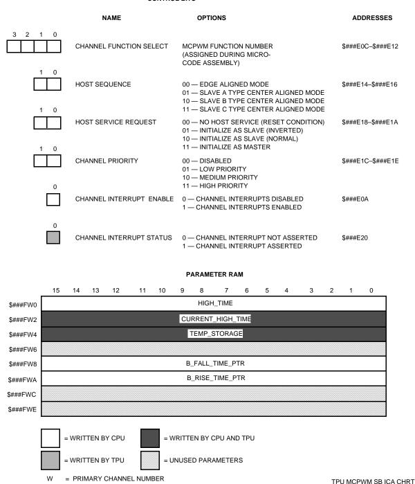
Figure D-18 MCPWM Parameters — Slave Ch B Inverted Center-Aligned Mode
