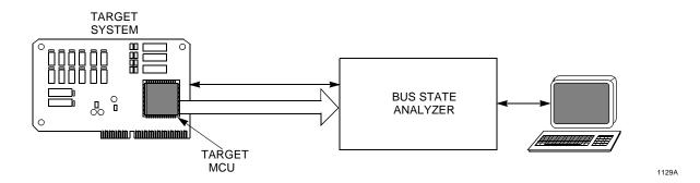
Figure 3-9 Bus State Analyzer Configuration
