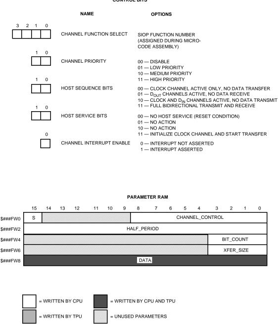
Figure D-28 SIOP Parameters
