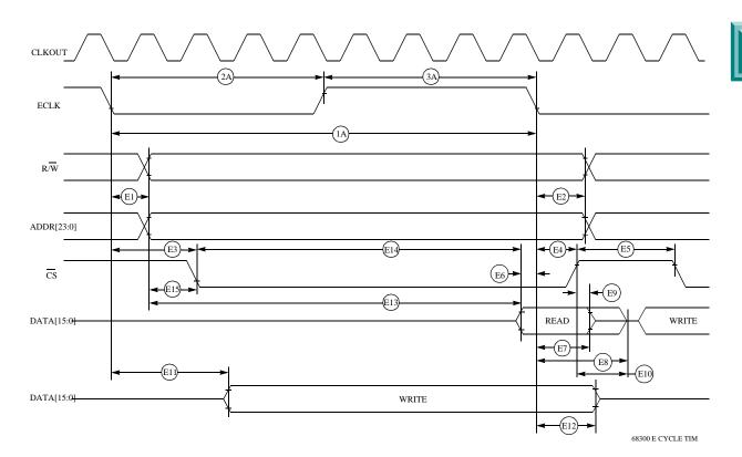
Figure E-15 ECLK Timing Diagram
