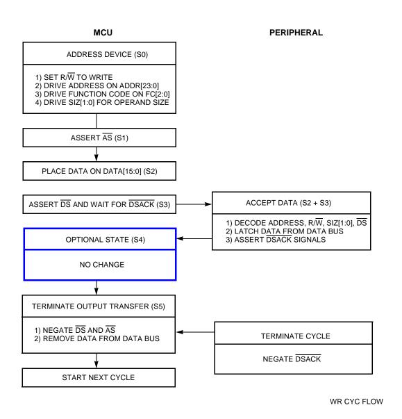
Figure 4-12 Write Cycle Flowchart
