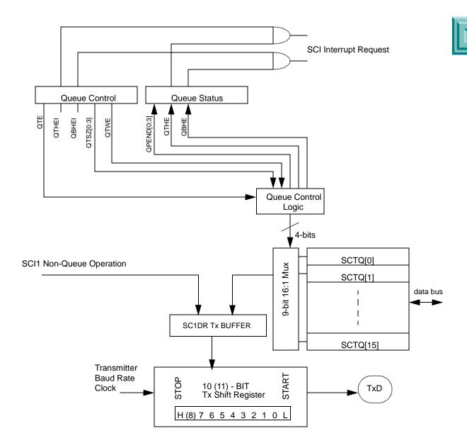
Figure 6-12 Queue Transmitter Block Enhancements
