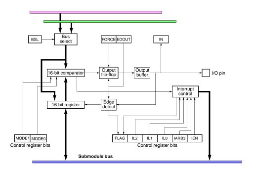
Figure 13-5 SASM Block Diagram (Channel A)
