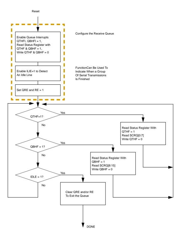
Figure 6-19 Queue Receive Software Flow
