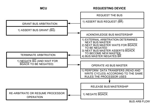
Figure 4-16 Bus Arbitration Flowchart for Single Request
