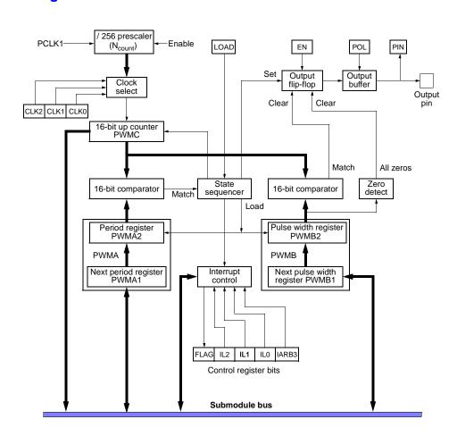
Figure 13-13 Pulse Width Modulation Submodule Block Diagram
