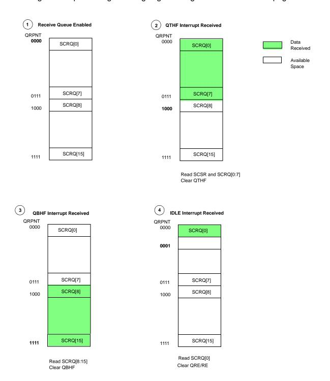
Figure 6-20 Queue Receive Example for 17 Data Bytes
