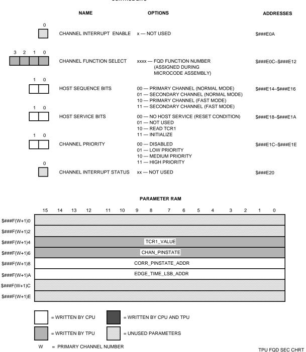
Figure D-20 FQD Parameters — Secondary Channel
