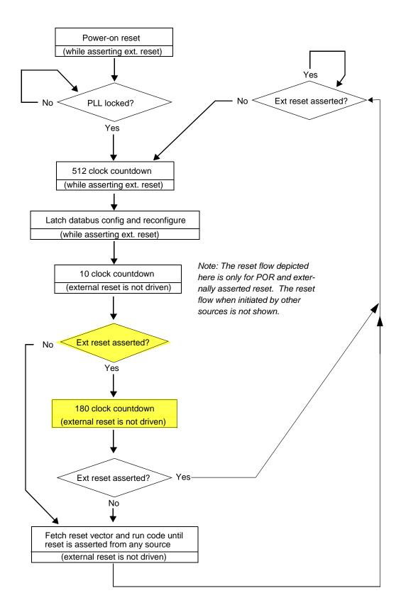
Figure 4-17 SCIM2 Reset Control Flow
