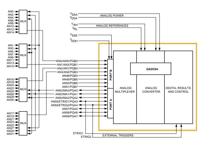
Figure 5-3 Example of Full External Multiplexing
