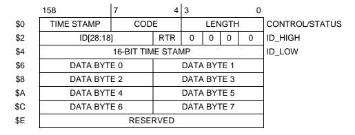
Figure 7-4 Standard ID Message Buffer Structure
