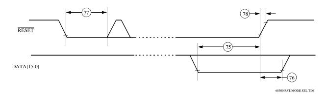
Figure E-12 Reset and Mode Select Timing Diagram
