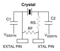
Slow Reference Mode (32.768 KHz): RF=1-10 m $\Omega$  RS=330 K $\Omega$ , C1=C2=22 pF Fast Reference Mode (4.194 MHz):RF=1-10 m $\Omega$  RS=1.5 K $\Omega$ , C1=C2=27 pF Fast Reference Mode (5.438 MHz):RF=1-10 m $\Omega$  RS=400  $\Omega$ . C1=C2=10 pF
