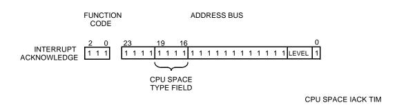
Figure 4-23 CPU Space Encoding for Interrupt Acknowledge
