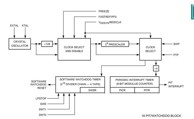
Figure 4-8 Periodic Interrupt Timer and Software Watchdog Timer
