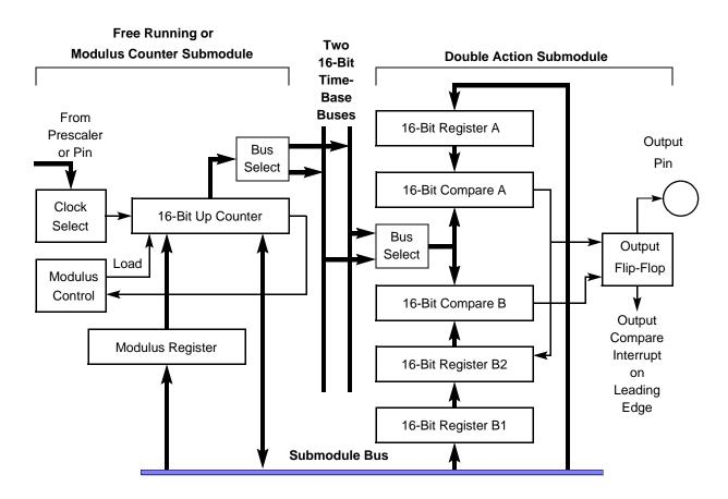
Figure 13-20 CTM9 Example — Pulse Width Modulation Output
