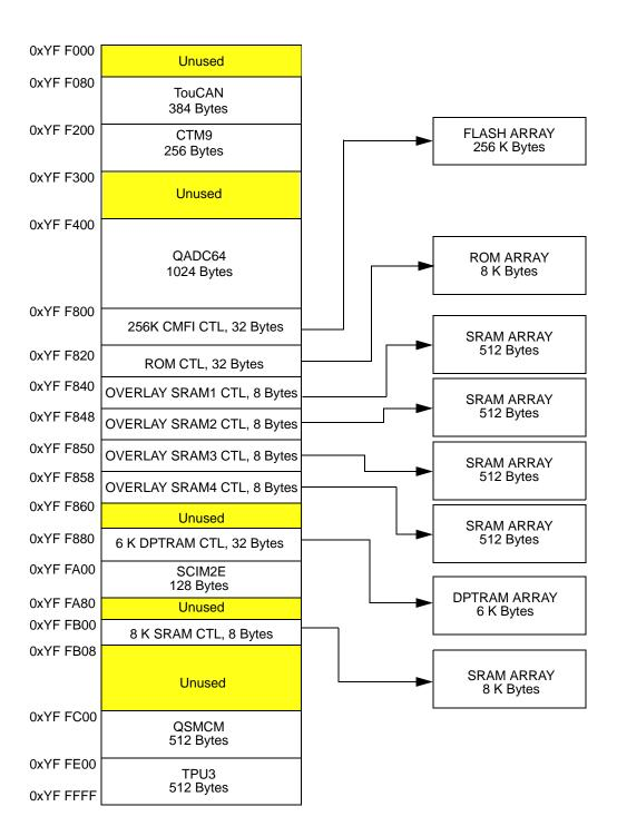
Y = M111, where M is the logic state of the module mapping (MM) bit in the SCIM2E configuration register (SCIMMCR).
