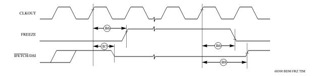
Figure E-14 Background Debugging Mode Timing — Freeze Assertion
