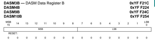
DASMB is the data register associated with channel B; its use varies with the different modes of operation. Depending on the mode selected, software access is to register B1 or register B2.
