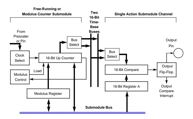
Figure 13-18 CTM9 Example — Single Edge Output Compare
