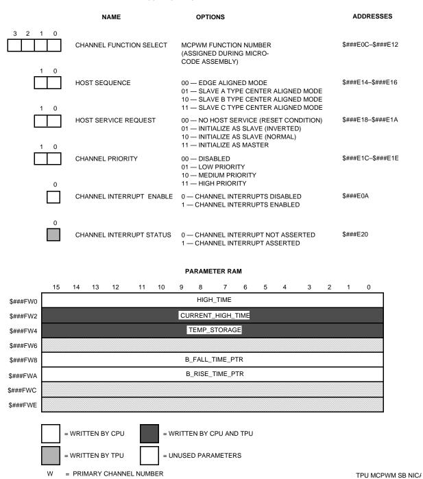
Figure D-16 MCPWM Parameters — Slave Ch B Non-Inverted Center-Aligned Mode
