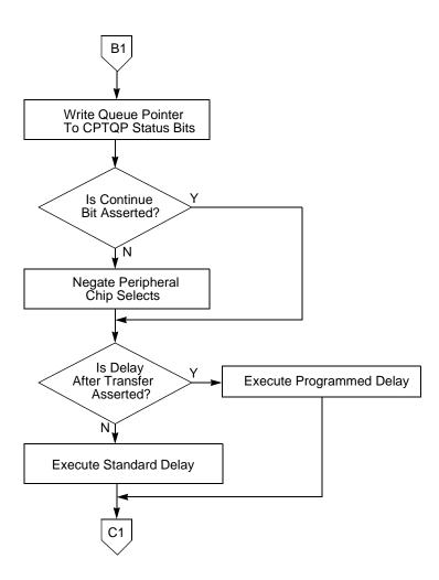
Figure 6-6 Flowchart of QSPI Master Operation (Part 2)
