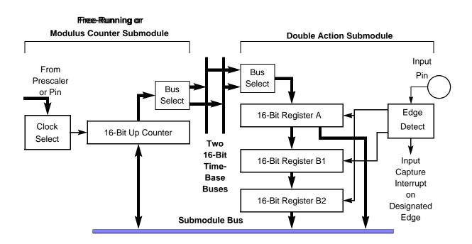
Figure 13-17 CTM9 Example — Double Capture Period Measurement
