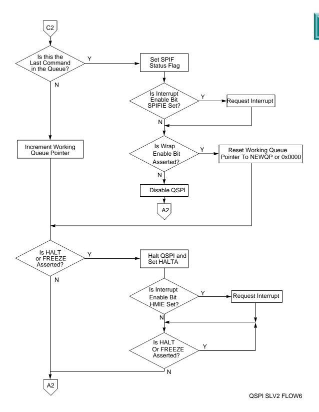
Figure 6-9 Flowchart of QSPI Slave Operation (Part 2)
