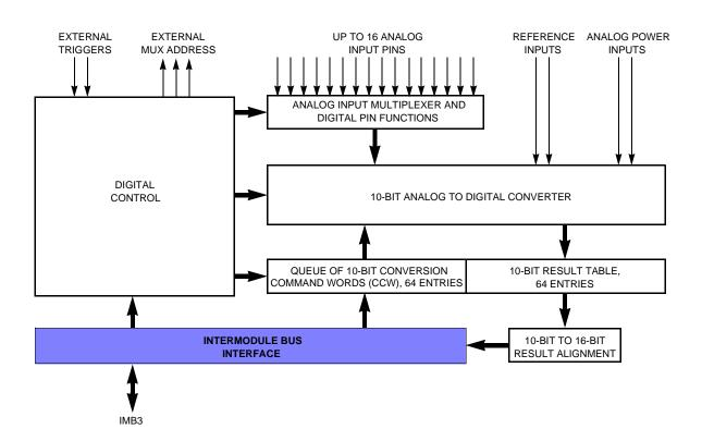
Figure 5-1 QADC64 Block Diagram
