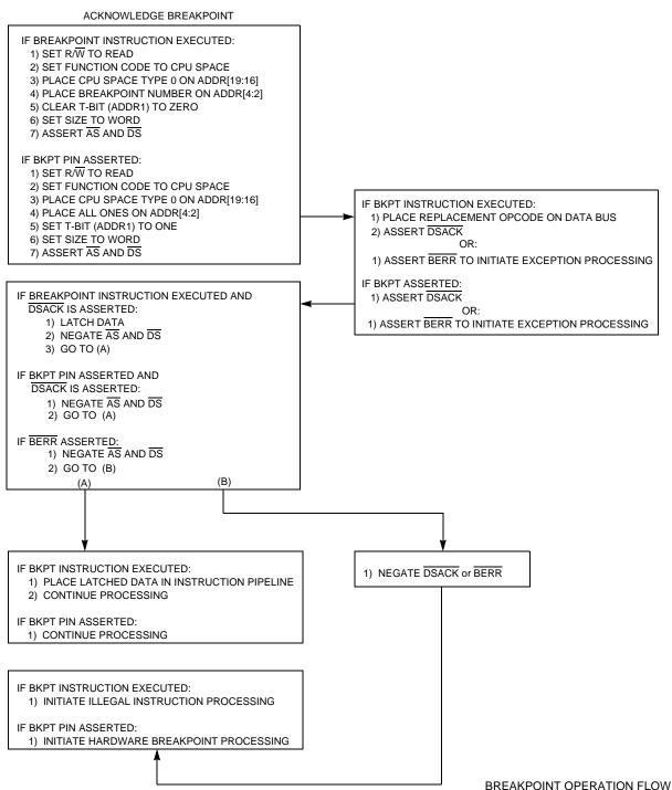
Figure 4-14 Breakpoint Operation Flowchart
