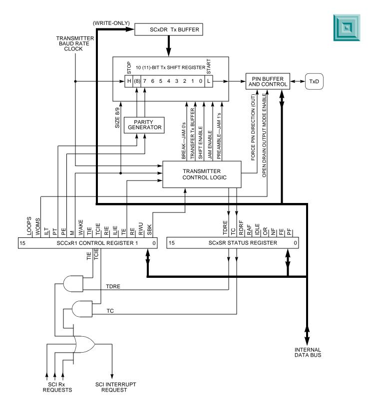
Figure 6-10 SCI Transmitter Block Diagram
