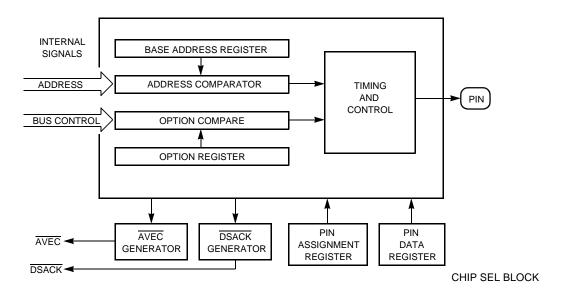
Figure 4-22 Chip-Select Circuit Block Diagram
