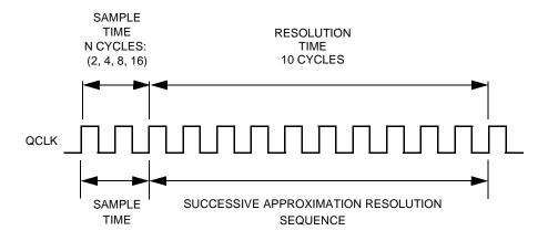
Figure 5-6 Bypass Mode Conversion Timing
