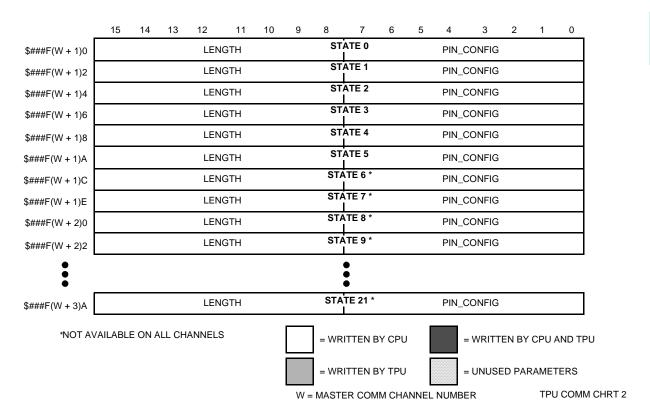
Figure D-11 COMM Parameters, Part 2 of 2
