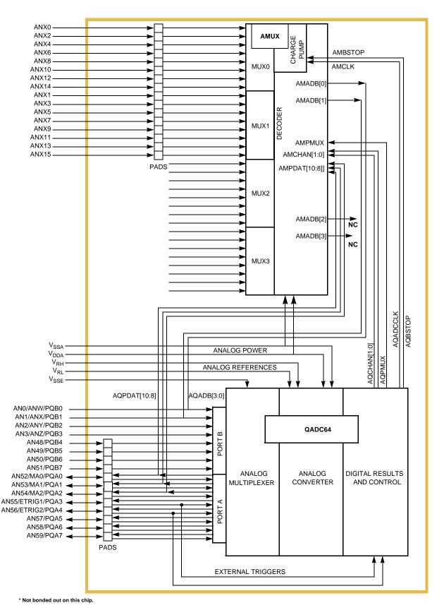
Figure 5-2 QADC64 Input and Output Signals
