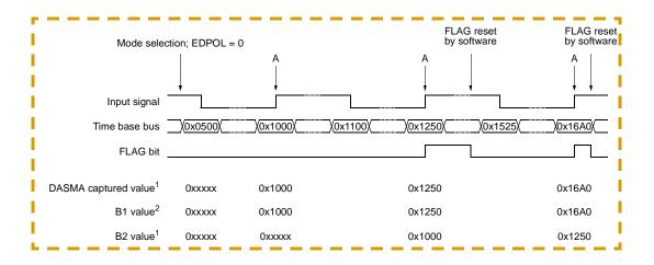
Figure 13-8 Input Period Measurement Example
