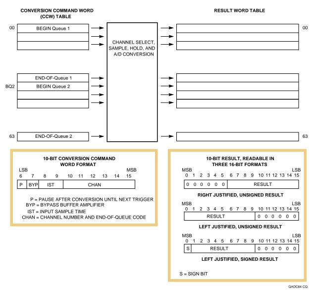
Figure 5-12 QADC64 Conversion Queue Operation
