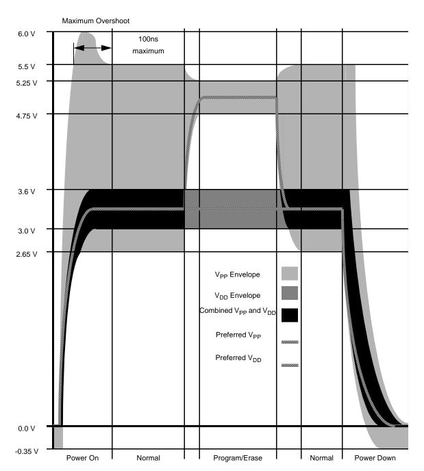
Figure E-22  $V_{PP}$  and  $V_{DD}$  Power Sequencing
