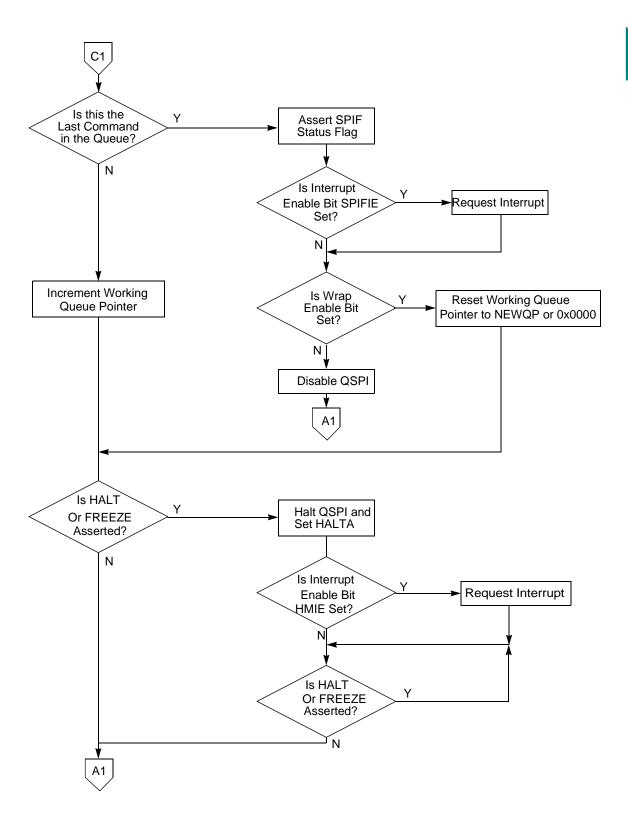
Figure 6-7 Flowchart of QSPI Master Operation (Part 3)
