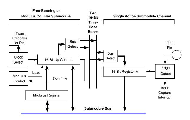
Figure 13-15 CTM9 Example — Single Edge Input Capture
