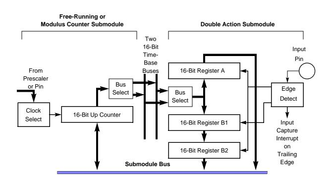
Figure 13-16 CTM9 Example — Double Capture Pulse Width Measurement
