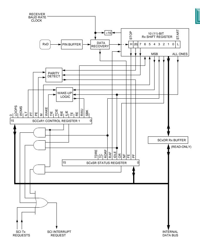
Figure 6-11 SCI Receiver Block Diagram
