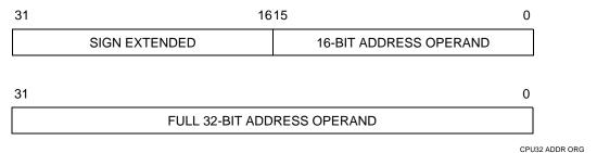
Figure 3-5 Address Organization in Address Registers
