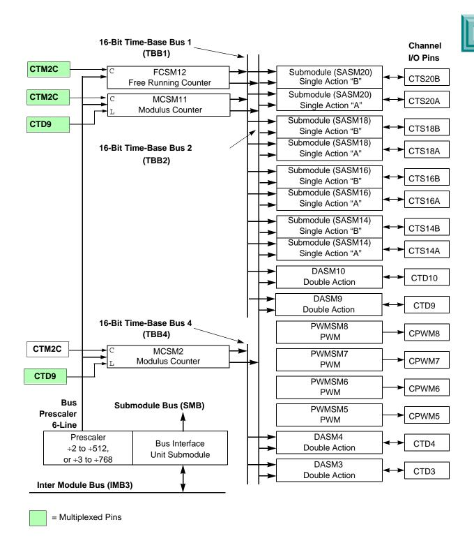
Figure 13-1 Configurable Timer Module, CTM9 Block Diagram
