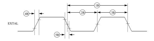
NOTE: TIMING SHOWN WITH RESPECT TO 20% AND 70%  $\rm V_{DD}.$  PULSE WIDTH SHOWN WITH RESPECT TO 50%  $\rm V_{DD}.$
