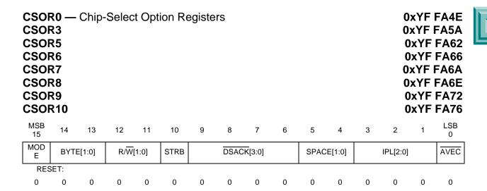
CSORBT and CSOR[0], [3] and [5:10] contain parameters that support operations from external memory devices. Bit and field definitions for CSORBT and CSOR[0], [3] and [5:10] are the same.
