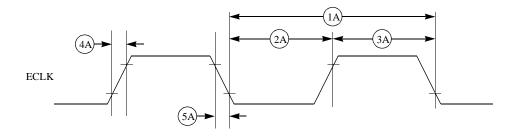
NOTE: TIMING SHOWN WITH RESPECT TO 20% AND 70%  $\rm\,V_{DD}$
