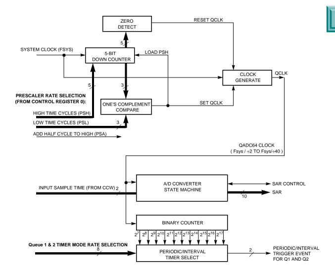
Figure 5-8 QADC64 Clock Subsystem Functions
