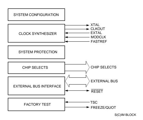
Figure 4-1 SCIM2E Block Diagram
