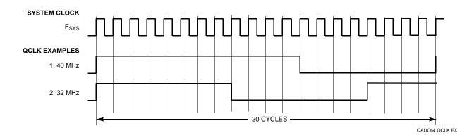
Figure 5-9 QADC64 Clock Programmability Examples
