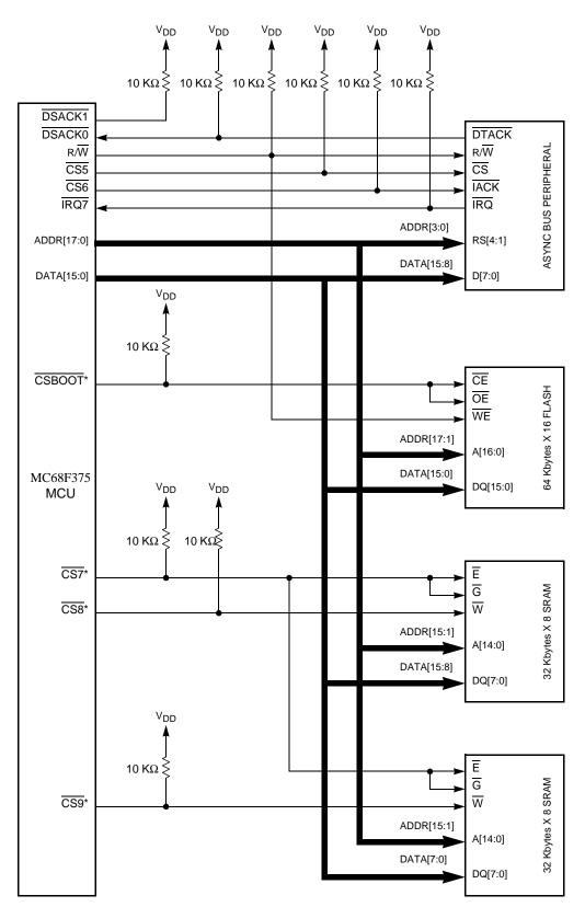
1. THESE CHIP-SELECT LINES ARE CONFIGURED FOR 16-BIT PORT OPERATION IN THIS EXAMPLE.
