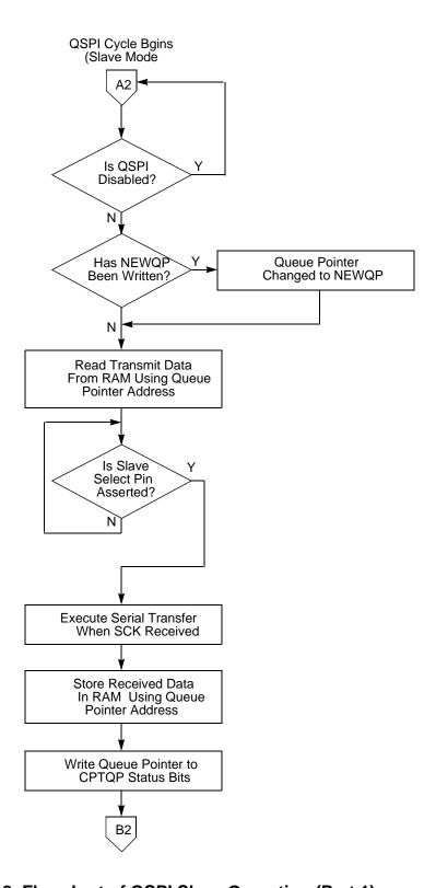
Figure 6-8 Flowchart of QSPI Slave Operation (Part 1)
