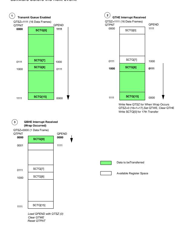
Figure 6-15 Queue Transmit Example for 17 Data Bytes
