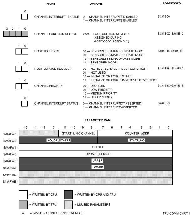
Figure D-10 COMM Parameters, Part 1 of 2
