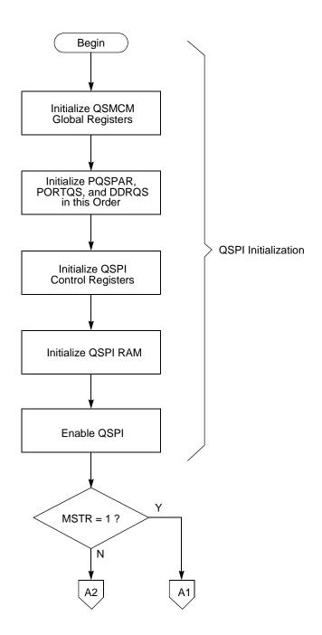
Figure 6-4 Flowchart of QSPI Initialization Operation
