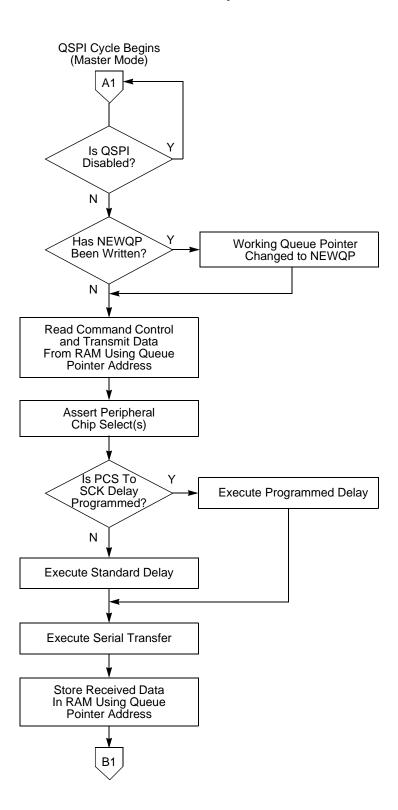
Figure 6-5 Flowchart of QSPI Master Operation (Part 1)
