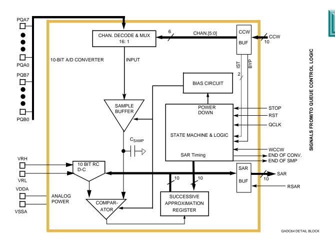
Figure 5-4 QADC64 Module Block Diagram
