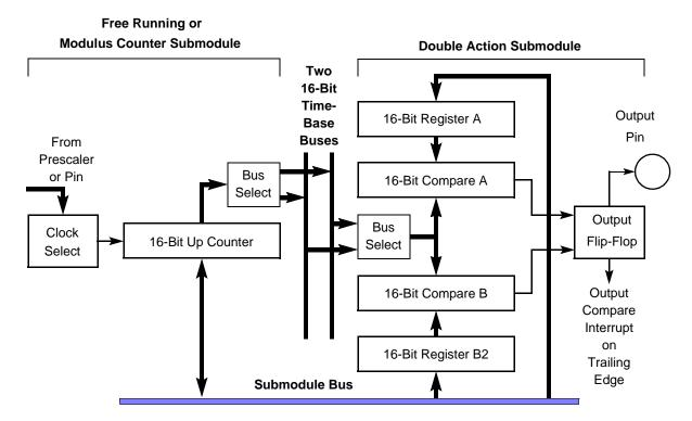
Figure 13-19 CTM9 Example — Double Edge Output Compare
