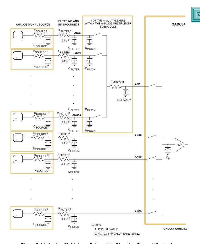
Figure 5-14 Analog Multiplexer Submodule Charging Current Illustration
