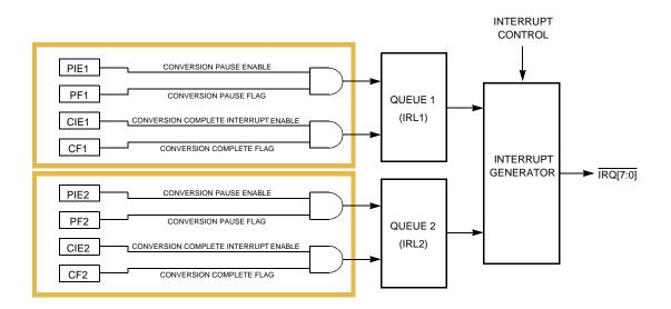
Figure 5-10 QADC64 Interrupt Flow Diagram
