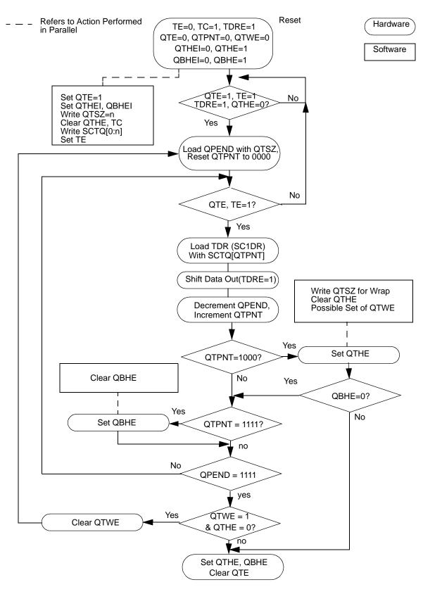
Figure 6-13 Queue Transmit Flow
